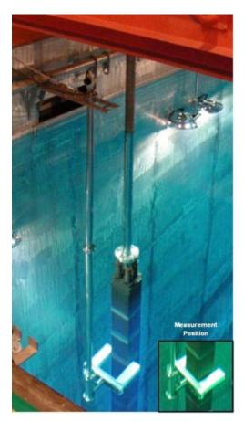
A Fork detector measuring a spent fuel assembly at a reactor pond. Photo credit: IAEA
