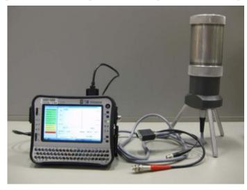
Miniature multichannel analyzer with NaI detector and portable computer. Photo credit: IAEA
