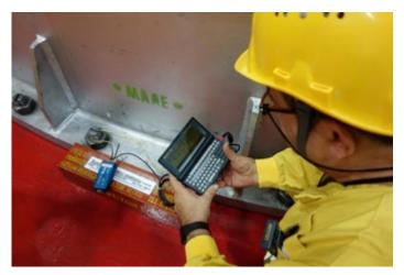
A VACOSS seal being attached by an IAEA inspector to a reactor core lid Photo Credit: IAEA Imagebank
