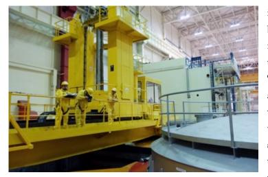
Inspectors at a bridge over a spent fuel pond verifying fuel assemblies with the ICVD. Photo credit: IAEA imagebank
