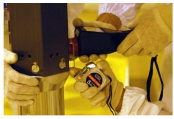
HM-5 spectrometer used for measuring the active length of a fuel assembly. Photo credit: IAEA imagebank
