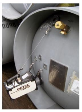
An electrically cooled germanium system used to verify the enrichment of UF<sub>6</sub>. Photo credit: IAEA imagebank
