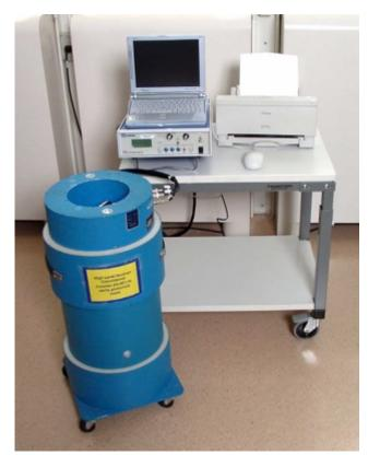
High-level neutron coincidence counter, HLNC, used to measure plutonium mass in combination with a determination of Pu isotopes. Photo credit: IAEA
