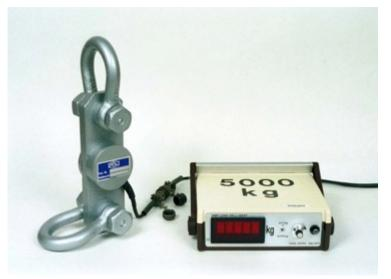
Load cell based weighing system with a capacity of 5000 Kg. Photo credit: IAEA
