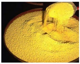
A drum with Yellow Cake being prepared for shipping to a conversion facility Photo Credit: Cameco/WNA reproduced with permission
