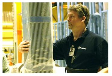
A PWR fuel assembly ready to be shipped to a reactor. Photo Credit: D. Calma, IAEA/Westinghouse Electric Sweden AB Fuel Fabrication Plant
