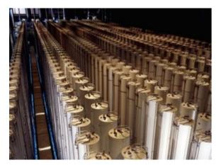
Cascade of gas centrifuges used to produce enriched uranium. Source: US DOE, Public Domain
